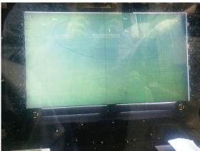
图 6 卡夹运输不良现象 Fig. 6 Defect phenomenon of cassette transportation
